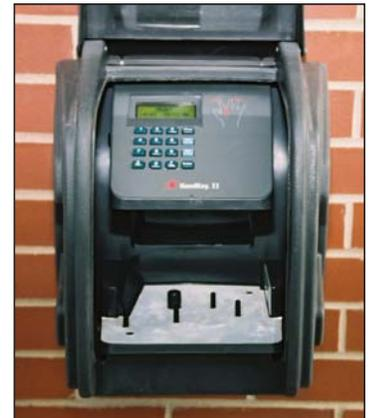
*Access to 67 secure doors and even the elevators is controlled with unique bio-readers providing three-dimensional hand scans.*
